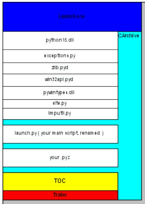
Fig. 3: Structure of the Self Extracting Executable
